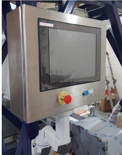
A smaller HMI located next to the box erector provides monitoring, setup, and diagnostics for the box erector.
