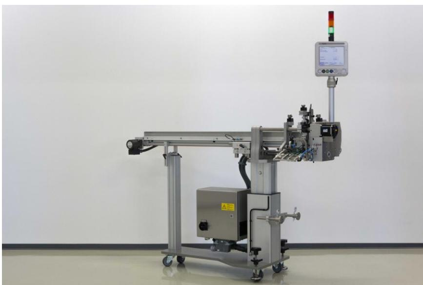
The feeder is positioned above the chain. The speed is synchronized by a rotary encoder, which is mounted on the chain.
