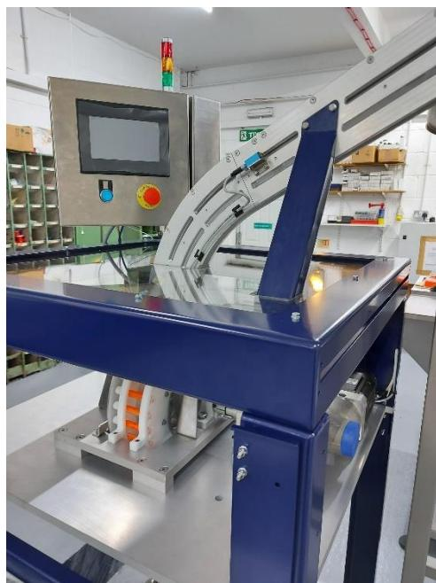
The tube delivery system consists of a bowl feeder and a rotating star wheel. Tubes are fed from the bowl feeder to the star wheel chute and deposited into each of the shrink wrap packed by the synchronised wheel.
